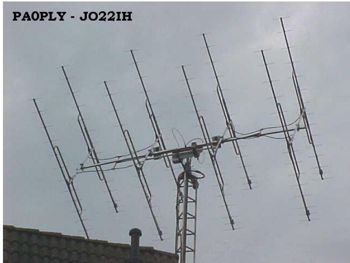
Photo 1.: Large EME array for 432MHz.
