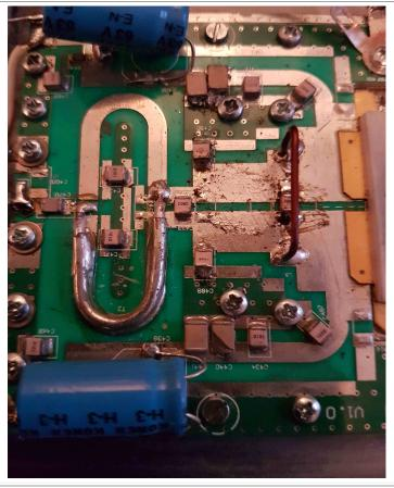
Initial tune up at low level: 0dBm input C426 = 6p8 C423 = 3p0 C489/490 = 3p0
