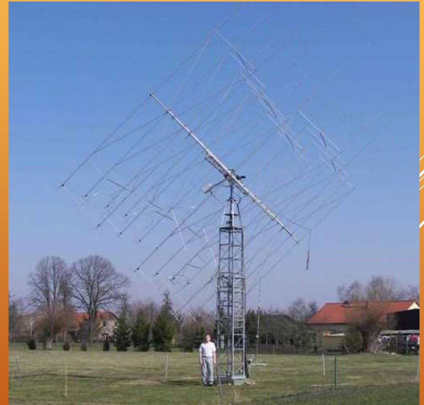
Antenna: 16 x 13 \lambda | DJ9BV Gain: 29.7dBD
