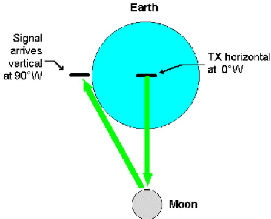
Geometric rotation also depends on the moon's position, so it varies with time on each moon pass. The graph below shows how geometric rotation can typically change, for two stations with a 6-hour local time difference.
