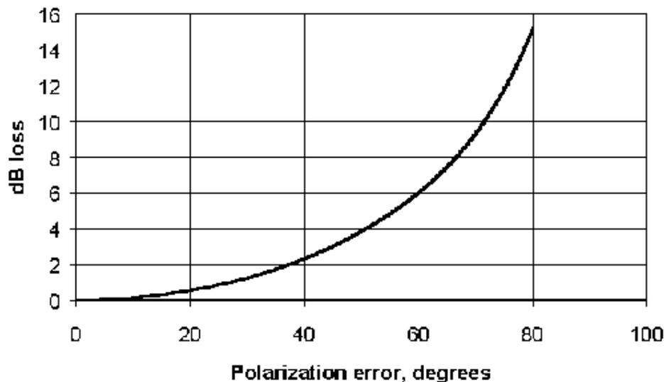
To keep the signal losses below 1dB, the polarization error must be less than about  $\pm(20-30)^\circ$ . The good news is that the signal loss within the  $\pm 20^\circ$  region is very small.
